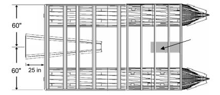
• If  $\frac{3}{4}$ " plywood and carpeting is used, the outside perimeter needs routing 1" wide x  $\frac{1}{8}$ " deep.
