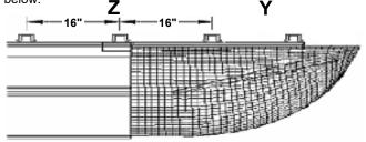
• The first two hat bars should be positioned as above for #A and #Z. The distance from the back of the riser to the center of #Z should be a multiple of the centers used e.g. 12" - 16" etc Note:hat bar #A is installed so that the outside of the lip is in line with the end of the risers.
