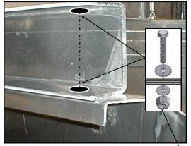
The spacers should be attached to the motor support first.
