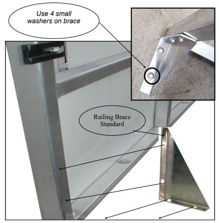
2. Once the railing is positioned on the deck the way you want it, drill the necessary 1/4" holes through the bottom horizontal square tube. (Page1)
